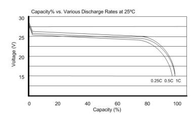
The rechargeable pbq LiFe battery employs lithium iron phosphate as its cathode and carbon as its anode.
