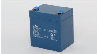
The rechargeable pbq LiFe battery employs lithium iron phosphate as its cathode and carbon as its anode. The electrolyte salt dissolves in organic compound solvent and the electrolyte system is absorbed by the separators and the plates. All batteries of this type have a special oneway valve to allow the disaggregate-tire solvent gases to escape.
