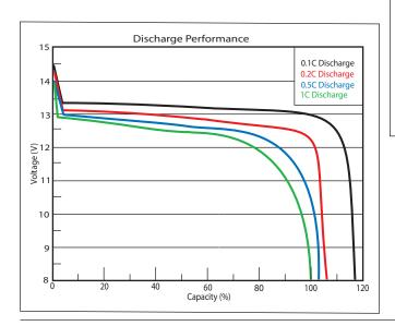
Each individual cell is spiral wound and formed to a prismatic cell. The nominal cell voltage is 3.2V. Four cells are placed in series in order to create 12.8V. To protect the battery from over charging and over discharging the battery is equiped with a internal battery management system (BMS). The BMS also takes care of
