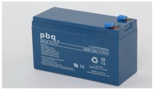
The rechargeable pbq LiFe battery employs lithium iron phosphate as its cathode and carbon as its anode. The electrolyte salt dissolves in organic compound solvent and the electrolyte system is absorbed by the separators and the plates. All batteries of this type have a special oneway valve to allow the disaggregate-tire solvent gases to escape.
