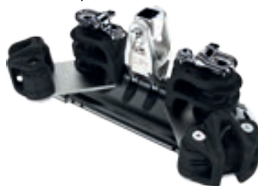
TB Car with Upstand, Double CL Sheaves, Becket & Cam (5:1)
