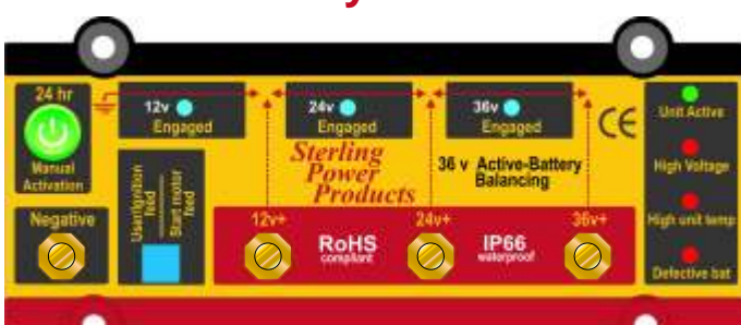
model shown, 36 volt 3 x 12 v battery bank
