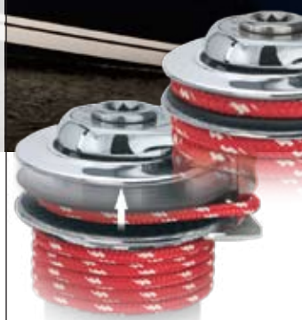
Self-tailing jaws accept a wide range of line sizes
