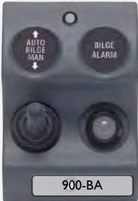
Bilge alarm and bilge pump control panel includes: 1 on/off/on switch for auto manual control; 1 warning light and alarm for high water level alarm. (Float switch ordered separately – Part No. SBI-FS)
