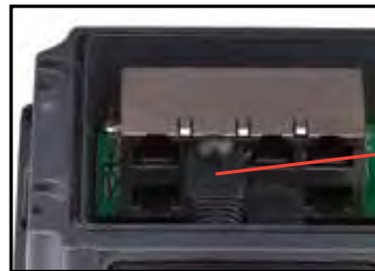
8-Way Connector Bank for SCI Cable Assembly to Switches
